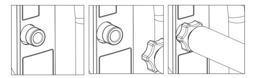
• Join the quick connect hose attachment to the air inlet on the spray gun. Tip: If connection is tight loosen the quick connect fitting on the hose by unscrewing a little before connecting to the gun, then retighten.
