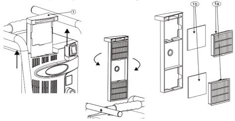
Check the condition of pre-filter (1b) carefully and replace if necessary. **WARNING!** Ensure filter is completely dry before installing.
